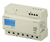
The COUNTIS E3x is a modular energy meter displaying the energy and power consumed (kWh and kW) directly on its backlit LCD display. It is designed for threephase load metering and is used for direct connections of up to 100 A. COUNTIS E32, E34 and E36 are also MID-certified.
